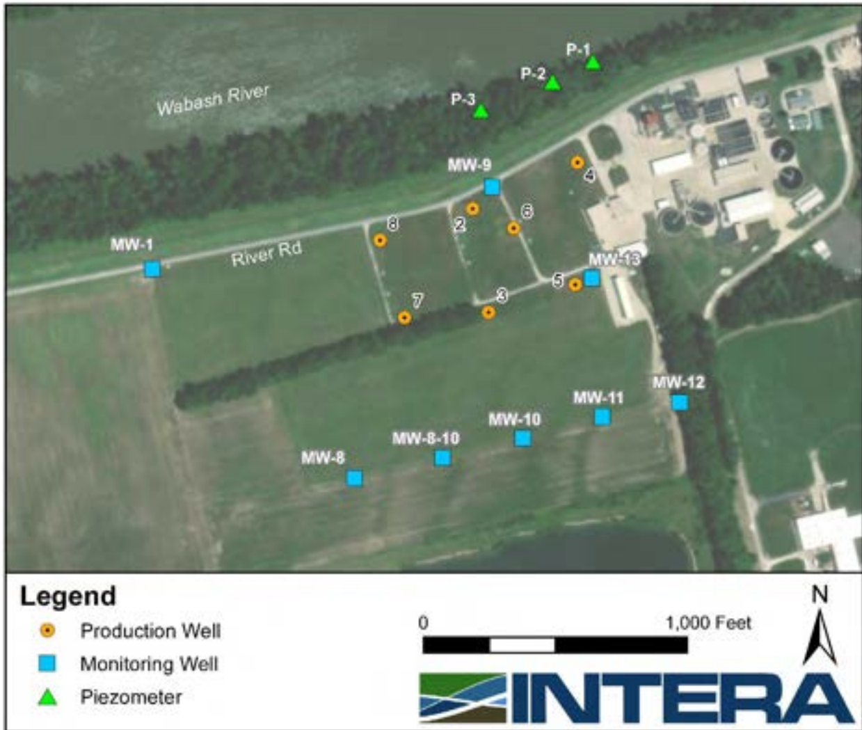
Figure 2: Monitoring locations near the VWU well field.
