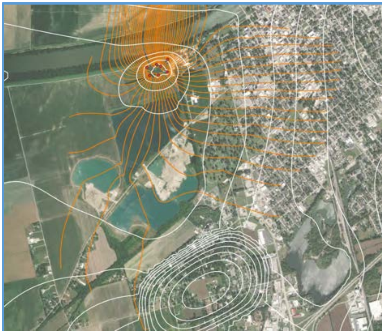
Figure 22: Pathlines traced backwards from the wells showing the interaction of the well field with the gravel pits to the south.
