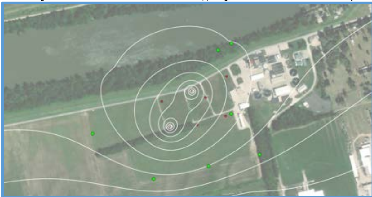
Figure 20: Local calibration to conditions observed on September 22, 2023, at midnight. Observation points are shown as green circles. Piezometers P1 and P2 are in the upper right-hand corner. Contour interval is 1 foot.
